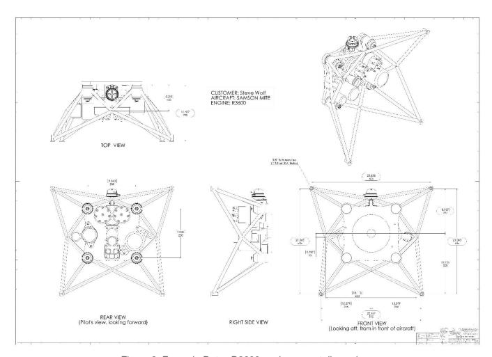
Figure 3: Example Rotec R3600 engine mount dimensions
